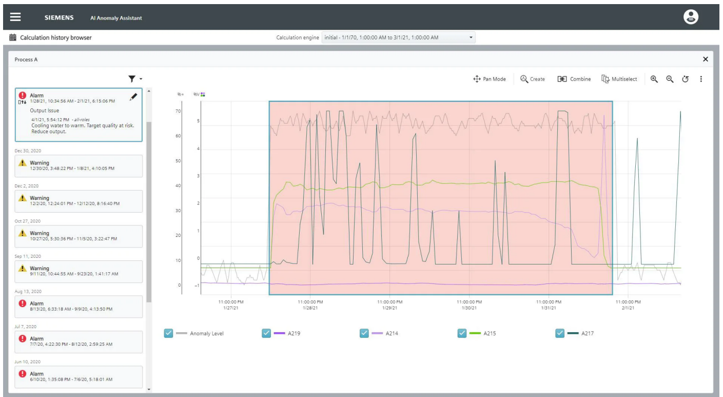
The AI Anomaly Assistant App uses artificial intelligence (AI) to detect anomalies in the process industry and assess their business relevance. A dashboard helps users classify and evaluate events.
